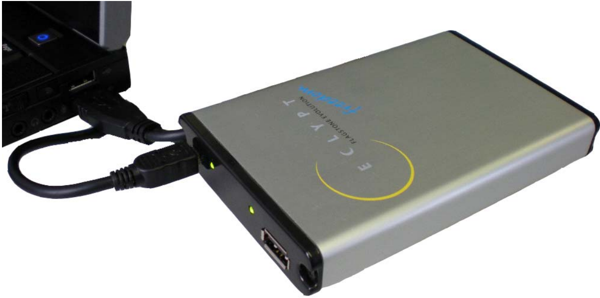
View of ECLYPT FREEDOM HMG Drive showing USB Connection to PC.
